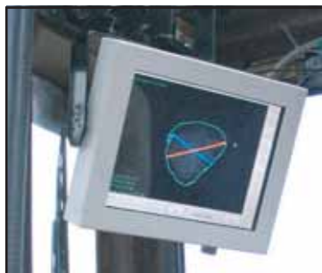
PictureTally for Logs system includes an industrial touch-screen mounted inside the cab for the operator's comfort and convenience.
