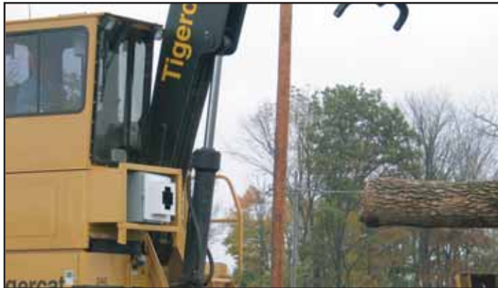
The PictureTally camera and control equipment (in white) are mounted on the outside of the cab in a weather-proof enclosure.
